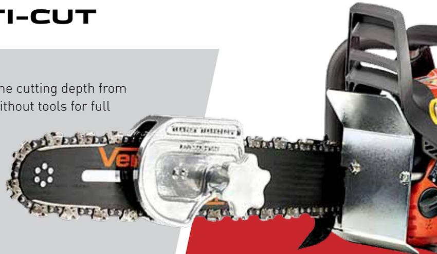
The conversion kit consists of a guide bar, the depth gauge (tool-less), a muffler deflector guard, a sprocket and the special chain. Optional: Full-wrap handle.
